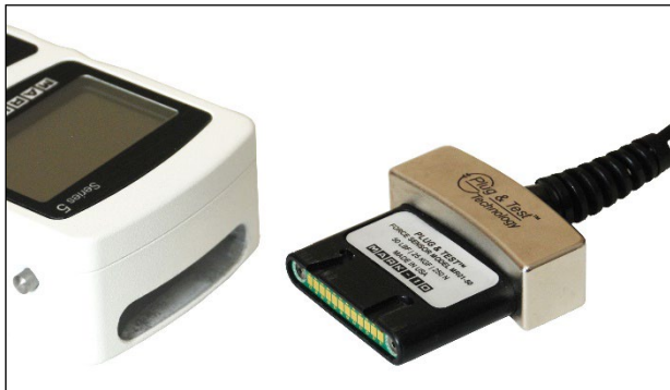
Fig. 3.1 Appropriate orientation of the Plug & Test® connector.
