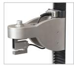
Install the sensor to the underside of the crosshead using the supplied socket head screw and hardware. Plug the connector into the connector into the receptacle in the top front surface of the crosshead, then fasten the two thumbscrews, as shown at left. Grips and fixtures may be threaded onto the underside of the sensor.
