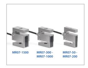
Series R07 force sensors measure tension and compression force, and are designed for use with Models F755, F755S, F1505, and F1505S test frames. Capacities available from 50 to 1,500 lbF [250 N to 7.5 kN]. Also compatible with Mark-10 indicators (sold separately) through unique Plug & Test® technology. Includes a certificate of calibration with data.
