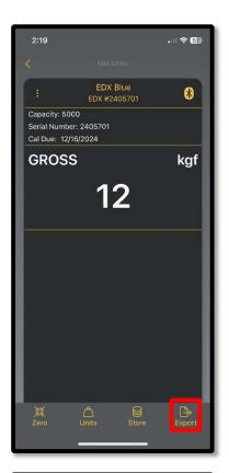
This will take you to a screen with the stored data page with the option to export as a PDF or Excel file. The logs will contain stored force readings with units and time stamps, as well as noting the unit's serial number, capacity, and calibration due date. Users can export the information in any format supported by the mobile device (email, airdrop, iMessage, text message, etc.)
